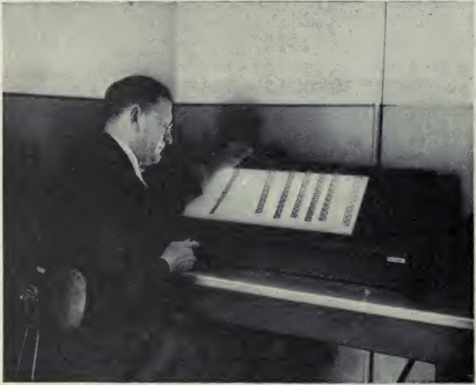
FIG. 6. The positive timer selects printer lights.
