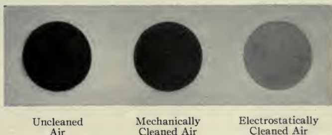
FIG. 2. Relative efficiency of air-cleaning methods (10,000 cu-ft of air through each sample).
