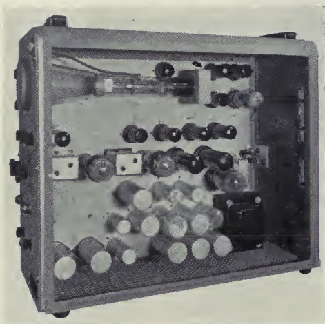
FIG. 14. Line amplifier, tube side.
